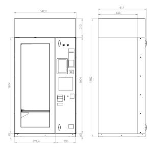
Width 1047,2 mm Depth 817 mm Height 1982 mm Weight (with 6 floors) 330 Kg Maximum number of floor 8 Maximum selections per floor 6 Lighting type High luminosity LED (25 W) 240/50 Hz | 110/60 Hz Power supply Indoor temperature -25 °C **Energy consumption** 900 W (with cooling unit on)
